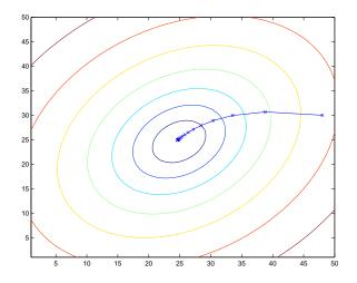
The ellipses shown above are the contours of a quadratic function. Also shown is the trajectory taken by gradient descent, which was initialized at (48,30). The x's in the figure (joined by straight lines) mark the successive values of  $\theta$  that gradient descent went through.
